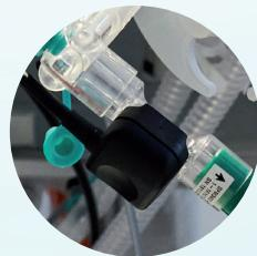
+ Heated electronic flow sensor
